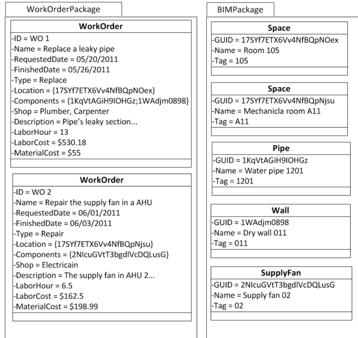
Figure 1 UML diagram of the instances of work orders and building elements for illustrating the implemented linkage between work order and BIM
